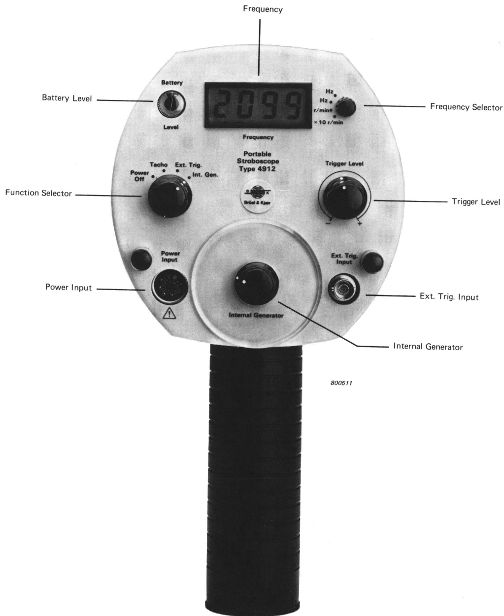
Fig.2.1. Rear panel of the 4912
